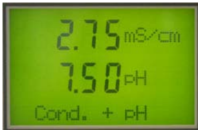
Simultaneous Conductivity and pH Measurement
