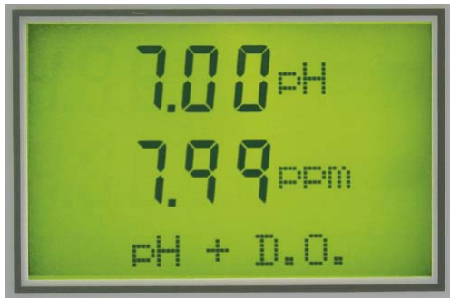
Simultaneous pH and Dissolved Oxygen Measurement
