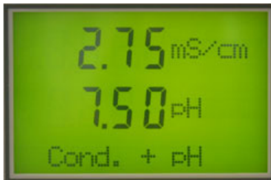
Simultaneous Conductivity and pH Measurement
