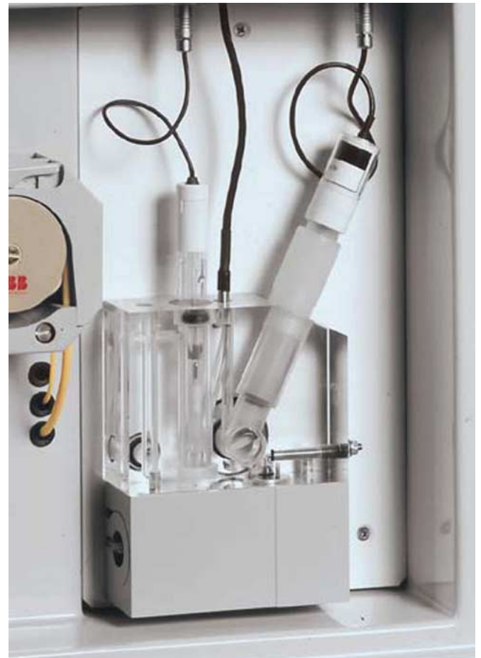
Multi-channel Peristaltic Pump and Sensor Flow Cell
