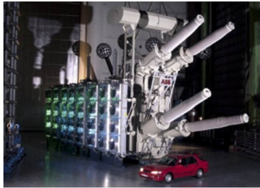
The 621 MVA converter transformer, 355 tons transport weight each.
