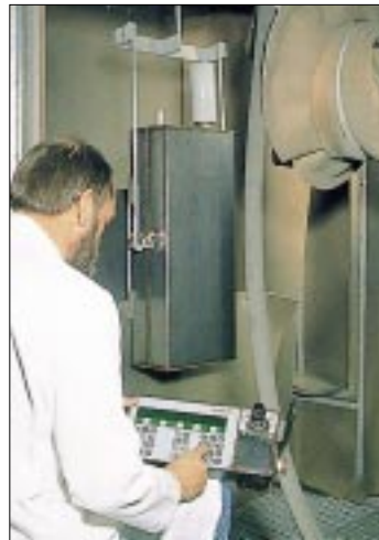
Programming of the blasting robot.
