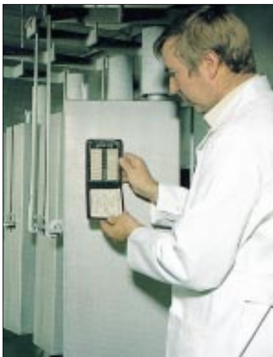
The degree of blasting is compared with a reference scale
