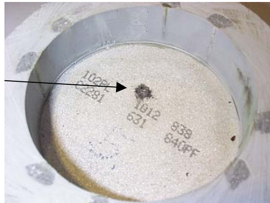
Fig. 6: Failure of a ZnO block due to TOV application. The block is punctured close to the centre. A silicone rubber insulator surrounds the ZnO block.
